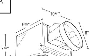
Acceptable for use over tub or shower when installed in a GFCI protected branch circuit.
