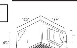
Acceptable for use over tub or shower when installed in a GFCI protected branch circuit.
