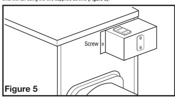
Plug the transformer from the motorized damper into the receptacle. Restore power and test the unit
