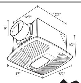
Acceptable for use over tub or shower when installed in a GFCI protected branch circuit.
